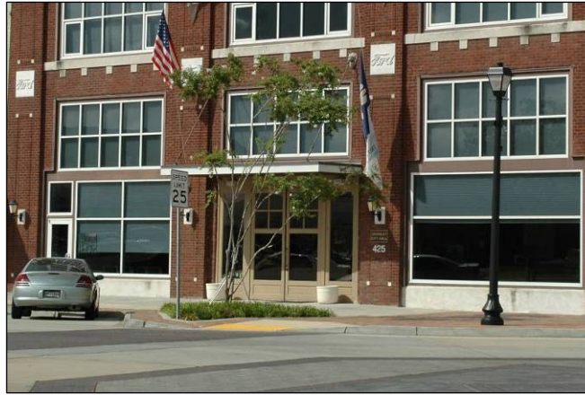
Windows flanking the door and sidelights maintain the proportions of the original automobile bays at this storefront.
